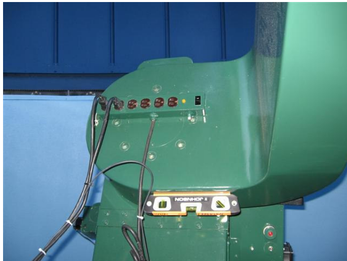
Figure 4: The upper part of the 24" telescope base. Note the fan/Telrad power supply and the right ascension bubble level.
