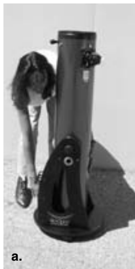
Figure 17. Picking up and carrying the SkyQuest IntelliScope as a single unit (with tube held captive on the base) requires some caution. (a) First, position the tube vertically. Then grasp the handle on the base with one hand while supporting the tube with the other. This ensures that the tube will not swing down and impact the ground (b) With knees bent, slowly lift the base while supporting the tube. (c) As you lift, continue to support the tube with one hand to keep it parallel with the ground. Make sure you are comfortable with the weight of the whole assembly before attempting the carry it!
