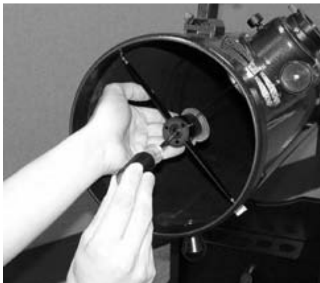
Figure 20. To center the secondary mirror under the focuser, hold the mirror holder in place with one hand while adjusting the center bolt with a Phillips screwdriver. Do not touch the mirror's surface!
